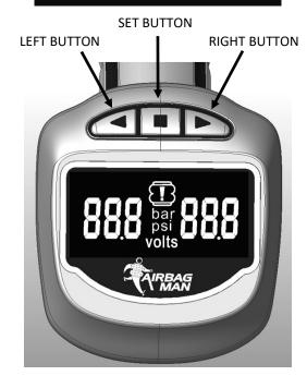
The display features Low and High pressure alarms. The display is supplied with the Low pressure alarm set at 5psi and the High pressure alarm set at 30psi. These pressure alarms can be set for your application.
